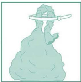
3. Pass the method of fastening (e.g. cable tie) over the twisted neck of the bag.
